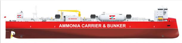
The "WorkHorse" as we have chosen to call this design, is an ammonia ship designed with added functionality for offshore bunkering of merchant vessels with ammonia propulsion. For these offshore bunkering operations, the vessel is equipped with high-capacity cargo pumps, motion-compensated loading arms, and dynamic positioning capabilities. Additionally, it features fenders with mooring winches, allowing vessels to be bunkered from both the portside and starboard side of the ship
